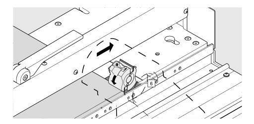
The depth stop [6] is used to position the workpiece. For workpieces with edge bands and for backs, we recommend using the timber stop [7].
