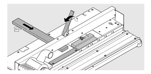
➤ Lay the back [31] on the base router, as shown.
