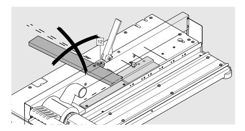
The support stop [12] must be aligned.
