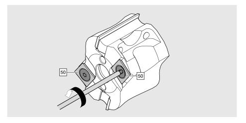
> Loosen the pre-cutter screw [50] by turning it anticlockwise.
