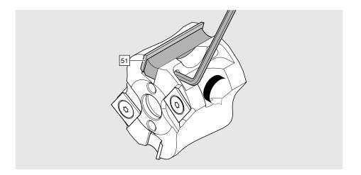
➤ Loosen the screw for the cutting insert [51] by turning it anticlockwise.
