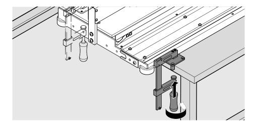
Secure the base router to the work top with fixing boards [1] and screw clamps.
