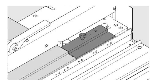
The timber stop [7] becomes worn through frequent milling. This can lead to torn edges on the workpiece. To avoid this, the timber stop [7] must be reworked, if necessary.
