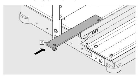
> Push the stop bar [13] into the runner of the base router.
