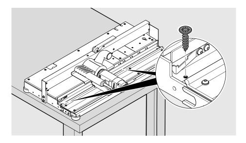
Screw the base router to the work top.
