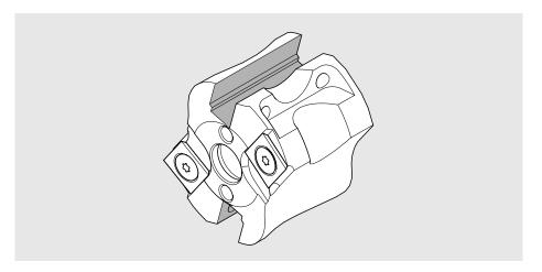
> Clean the base of the cutting inserts [51] using a dry cloth.
