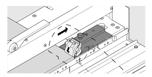
The timber stop [7] prevents torn edges and edge bands. When processing backs, the use of the timber stop [7] is strongly recommended.
