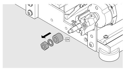
> Remove the spacer sleeve [24].
