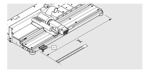
Position the fixing board [1] within the table length and screw to the frame.
