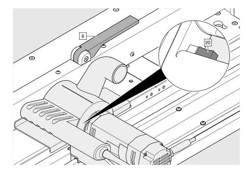
8 Clamping lever Press down the clamping lever [8] to secure the workpiece.
