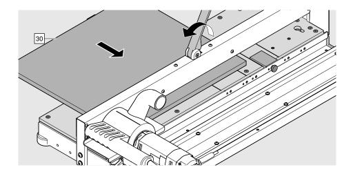
> Lay the drawer base [30] on the base router, as shown.
