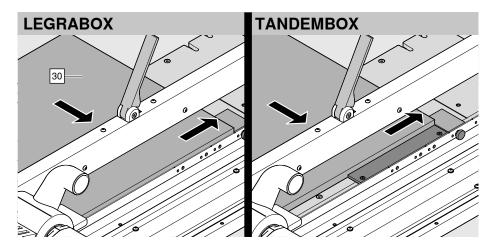
> Push the drawer base [30] onto the stops, as shown.
