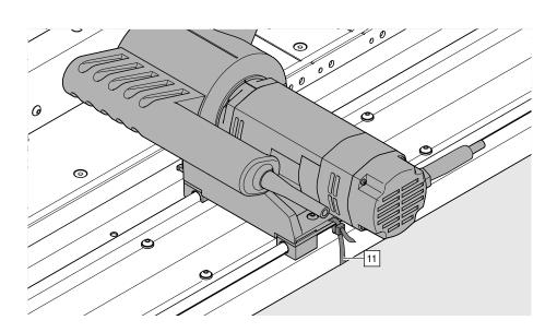
The carriage of the bottom router is secured for transport.
