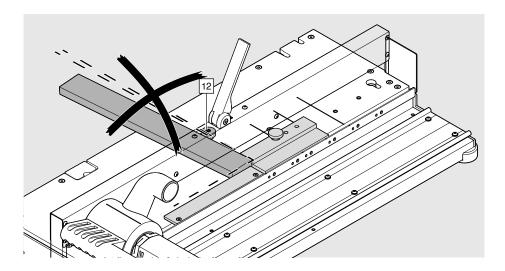
The support stop [12] must be aligned.
