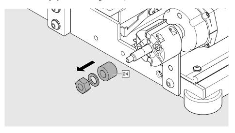
> Remove the spacer sleeve [24].
