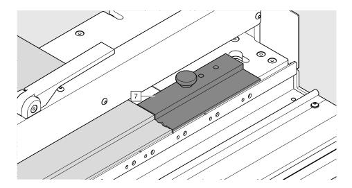
The wood stop [7] becomes worn through frequent routing. This can lead to torn edges on the work piece. To avoid this, the wood stop [7] must be reworked, if necessary.
