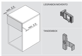
The front gap should be adjusted identically on each side to a minimum of 2.5 mm.
