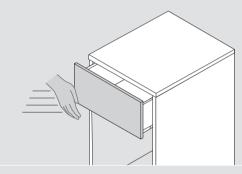
To tension TIP-ON springs, always close pull-outs with TIP-ON BLUMOTION with some force. Reduce the amount of force used accordingly for loaded pull-outs.
