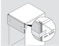
a) clamp an insert between front and cabinet or
