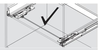
For optimal function and an optimised trigger range for TIP-ON BLUMOTION, use synchronisation linkage.
