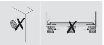
Do not use a bumper, as this restricts the triggering function. The cabinet bottom may not bend upwards, therefore do not use a fifth base leg.
