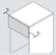
b) adjust the front gap to 0 mm or
