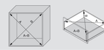
To ensure a front gap of at least 2.5 mm, precise manufacturing is required, so it should be ensured that planned measurements and angle accuracy are adhered to.
