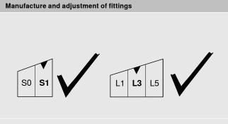
Select the right TIP-ON BLUMOTION unit: The marking on the underside shows the respective load configuration (for short nominal lengths S0 and S1, for longer nominal lengths L1, L3 and L5).
