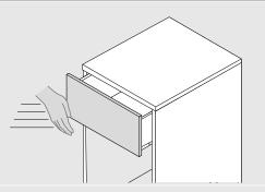
To tension TIP-ON springs, always close pull-outs with TIP-ON BLUMOTION with some force. Reduce the amount of force used accordingly for loaded pull-outs.
