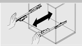
For LEGRABOX/MOVENTO: Open or close cabinet profiles with synchronisation in parallel, in order to prevent damage to the synchronisation adapter.
