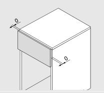
b) adjust the front gap to 0 mm or
