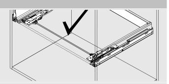
For optimal function and an optimised trigger range for TIP-ON BLUMOTION, use synchronisation linkage.
