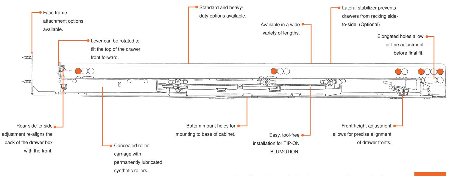
• Front side-to-side and optional depth adjustment available on locking devices.
