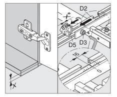
**b)** If the lower edge of the door is to be longer or shorter than the lower edge of the cabinet, the stops (D5) must be adjusted accordingly by the difference in dimension. In addition, the base ruler (D2) must be repositioned.
