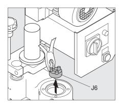
Lift the motor and rest it on the control system.
