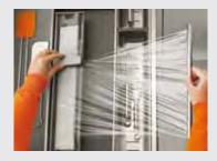
The cutter bar makes it easy to pull and cut film.
