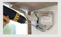
The lift mechanisms can be adjusted to the respective door weight using a cordless screwdriver.
