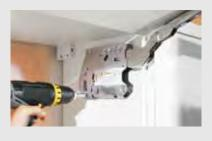
The lift mechanisms can be adjusted precisely to the corresponding door weight.
