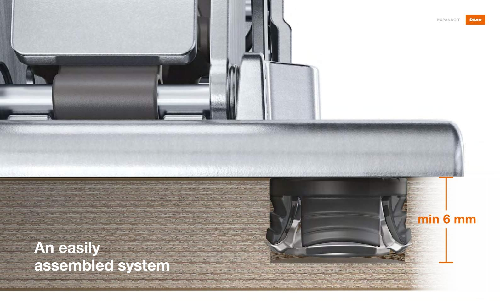
Our fixing system for thin fronts is based on EXPANDO T. Steel teeth bite into the material of hard fronts, and nylon components ensure firm anchorage in soft panels. To fix EXPANDO T, drill a hole of 10 mm in diameter and just 6 mm in depth.
