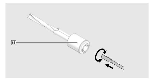
The length of the drill bit [83] can be adjusted.
