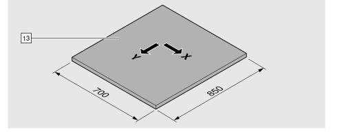
Larger work pieces [13] must have additional clamping, support and attachment. Small work pieces [13] that do not fit in the hold down clamps must be clamped using suitable means.
