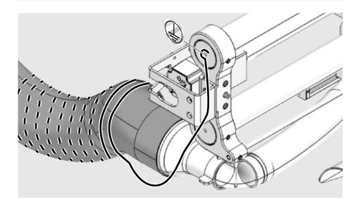
> Connect the spiral wire of the suction hose to the assembly machine.
