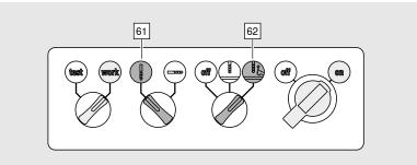
> Set the drilling mode selector switch [61] to vertical drilling.
