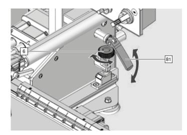
Height adjustment knob [6] for horizontal drilling. Drilling height adjustment range: 6 - 20 mm. A clamping lever [81] secures the setting.
