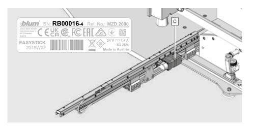
> Read off the serial number on the rating plate [C] of the EASYSTICK ruler.
