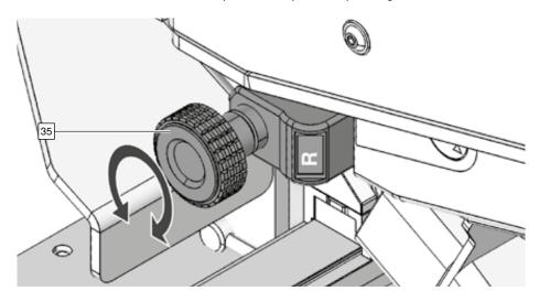
Set the residue material thickness [35].
