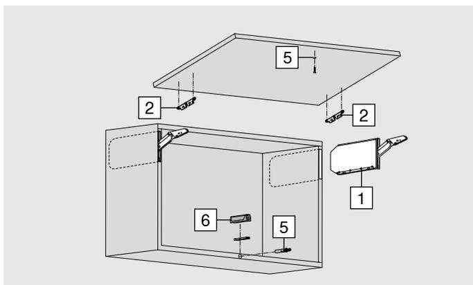
**Semi-integrated lift mechanism installation**
