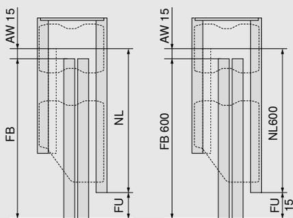
The minimum front protrusion results from the combination of nominal length, front width and the TIP-ON trigger path (AW) when using standard nominal lengths. By cutting the profiles to size, the front protrusion (FU) can be customised (min. FU = 7 mm).
