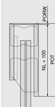
The depth requirement is the pocket depth (POT) and is determined by the nominal length + 100 mm, plus the pocket back.
