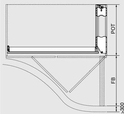
A minimum distance to the nearest element in front of the pocket must be kept free for safety reasons: front width + at least 300 mm
