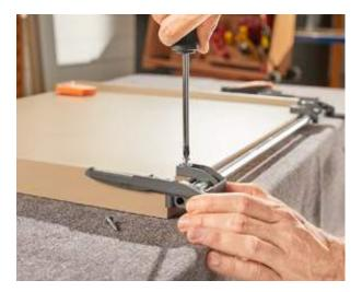
Locking unit and synchronisation shaft Attach the locking unit to the synchronisation shaft. It has to be flush with the pull-out shelf.
