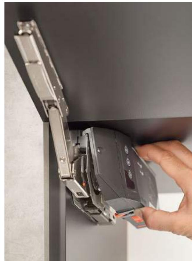
The new **SERVO-DRIVE for AVENTOS HK top** lift system is small in size but huge in functionality. Thanks to the CLIP mechanism, the drive unit can simply be clipped onto the AVENTOS HK top lift mechanism without tools.
