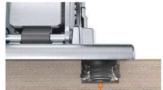
Steel teeth bite into the material of hard fronts, and nylon components ensure firm anchorage in soft panels. To fix EXPANDO T, drill a hole of 10 mm in diameter and just 6 mm in depth.
