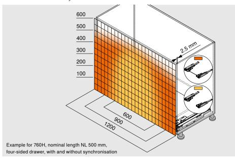
An extensive trigger range is achieved even with a low minimum front gap of 2.5 mm. To achieve optimal function and to extend the trigger range, we recommend using a synchronisation linkage.
