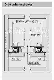
\*\* Limited side adjustment for a drawer side panel thickness of 16 mm, but with full tolerance utilisation of the internal drawer width
