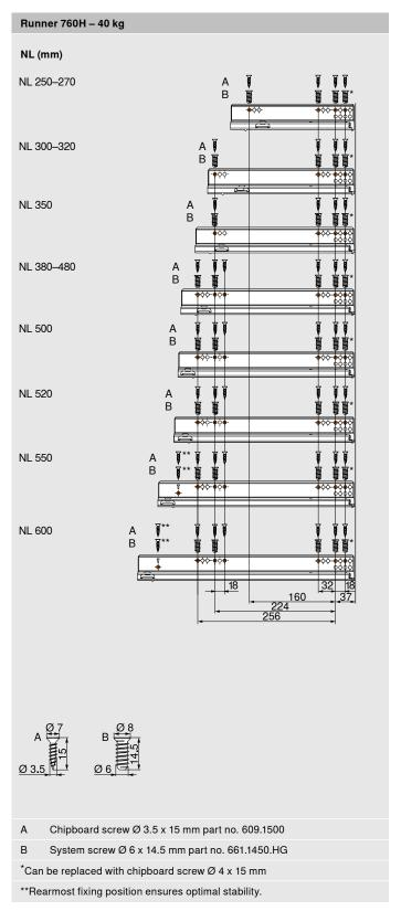
NL (mm) NL 450 NL 500 NL 520 NL 550 NL 580 NL 600 NL 650 NL 700 NL 750 \_\_18 320 416 Chipboard screw Ø 3.5 x 15 mm part no. 609.1500 Α В System screw Ø 6 x 14.5 mm part no. 661.1450.HG  $^{\star}$ Can be replaced with chipboard screw Ø 4 x 15 mm
