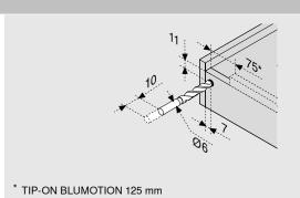
SKW Internal drawer width X Front thickness
