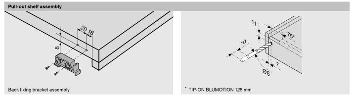
LTW Internal pull-out shelf width LW Internal cabinet width
