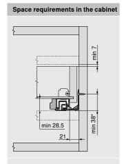
\* + 1 mm for assembly of the runners prior to cabinet assembly
