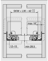
\* Limited side adjustment for a drawer side panel thickness of 16 mm, but with full tolerance utilisation of the internal drawer width
