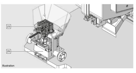
> Install the insertion ram [23] on the drilling head [25].
