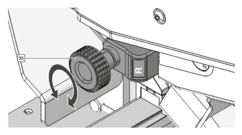
Set the residue material thickness [35].
