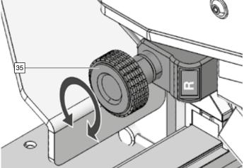
Residue material thickness adjustment knob [35]: Adjustment range: 2 - 37 mm
