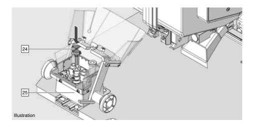
Clamp the drill bit [24] in the drilling head [25].
