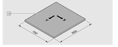
Larger work pieces [13] must have additional clamping, support and attachment. Small work pieces [13] that do not fit in the hold down clamps must be clamped using suitable means.
