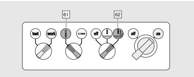
> Set the drilling mode selector switch [61] to vertical drilling.
