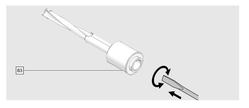
The length of the drill bit [83] can be adjusted.
