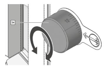
Board thickness adjustment knob [34] Setting the board thickness also sets the brake point (rapid speed/creep speed).
