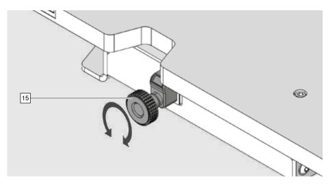
> Set the desired depth of the horizontal drilling via the hand wheel [15].
