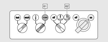
> Set the drilling mode selector switch [61] to horizontal drilling.
