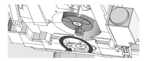
View of the coupling [K] from below: Coupling [K] direction of rotation: anti-clockwise.
