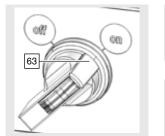
The main switch does not disconnect the assembly machine from the mains. Please note that the main switch does not disconnect the assembly machine from the pressurised air. No pneumatic motion is possible due to the use of solenoid valves.
