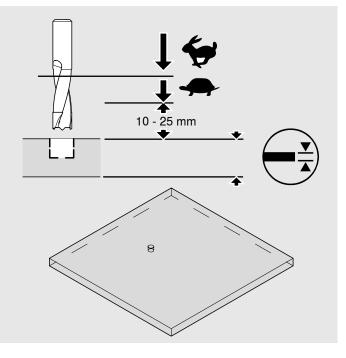
The creep speed can be set using this revolving knob [33].
