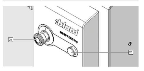
> Press the start button [20] until the drilling process is ended automatically.
