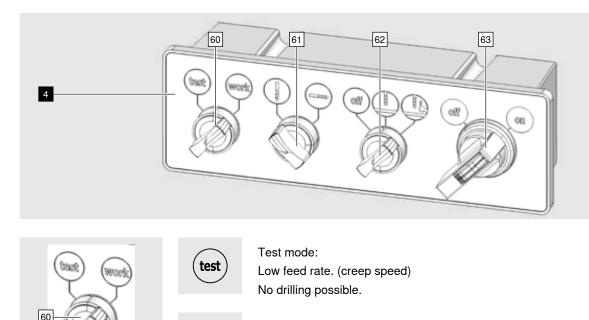
Work mode: Normal feed rate Vertical and horizontal drilling possible.
