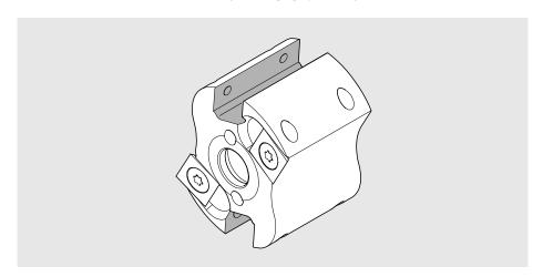
> Clean the base of the cutting inserts [51] using a dry cloth.
