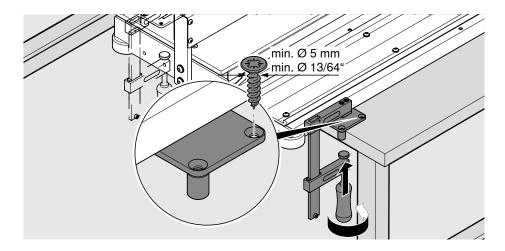
> Secure the bottom router to the work top with fixing boards [1] and screw clamps.
