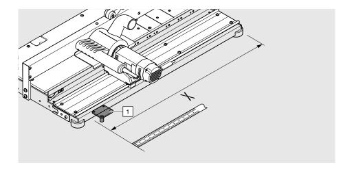
Position the fixing board [1] within the table length and screw to the frame.
