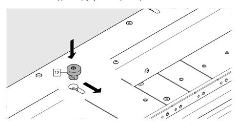
Mount the support stop [12] in the working position.
