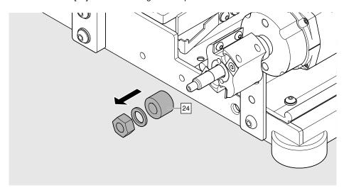
> Remove the spacer sleeve [24].
