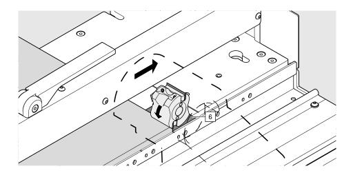
The depth stop [6] is used to position the work piece. For work pieces with edge bands and for backs, we recommend using the wood stop [7].
