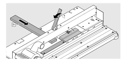
> Lay the back [31] on the bottom router, as shown.
