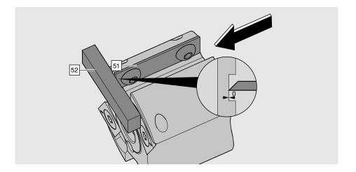
> Position the cutting insert [51] using the setting gauge [52].
