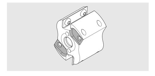
Clean the base of the pre-cutter [50] using a dry cloth.
