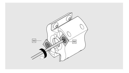
> Tighten the screw in the pre-cutter [50] by turning it clockwise.
