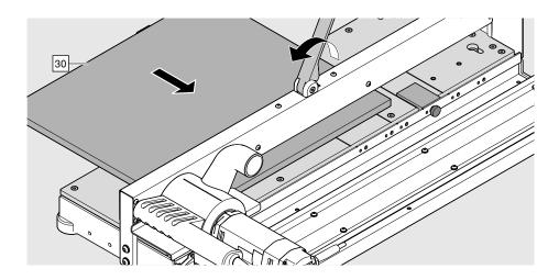
> Lay the drawer bottom [30] on the bottom router, as shown.
