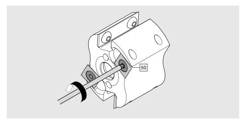
> Loosen the pre-cutter screw [50] by turning it counter clockwise.
