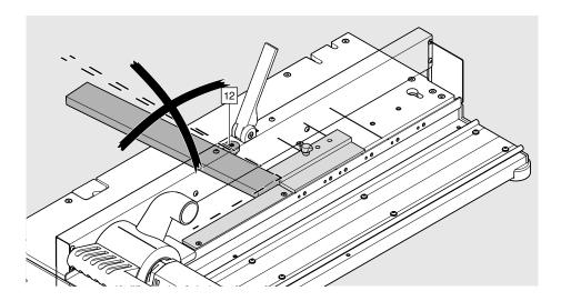
The support stop [12] must be aligned.
