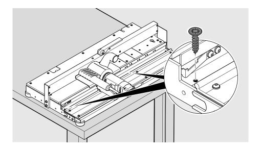
Screw the bottom router to the work top.
