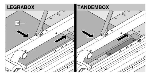
> Push the drawer bottom [30] onto the stops, as shown.
