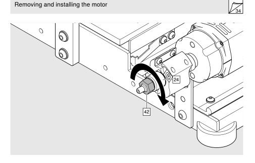
> Turn the nut [42] clockwise using the IM spanner.
