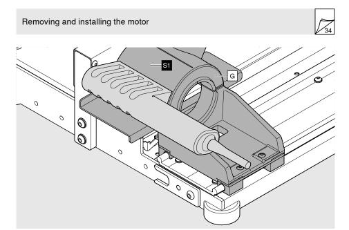
Remove the wood chips from the housing [G].
