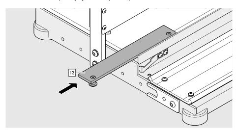
> Push the stop bar [13] into the runner of the bottom router.
