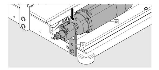
> Place the motor [40] in the shaft holder [2].
