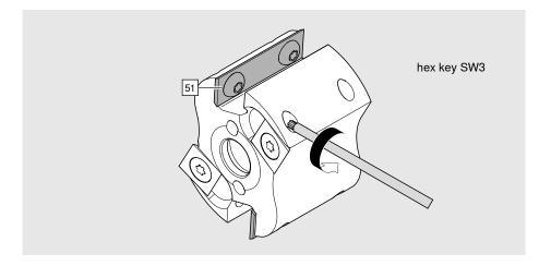
> Loosen the screw for the cutting insert [51] by turning it counter clockwise.
