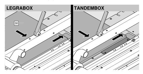
> Push the drawer bottom [30] onto the stops, as shown.
