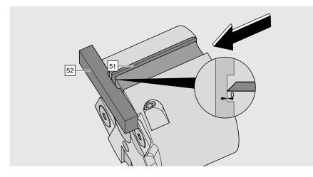
> Position the cutting insert [51] using the setting gauge [52].
