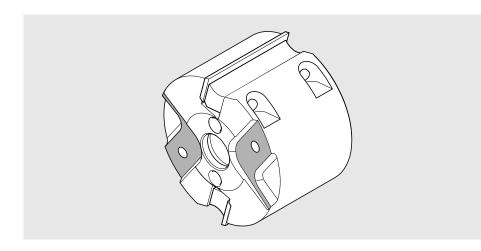
> Clean the base of the pre-cutter [50] using a dry cloth.
