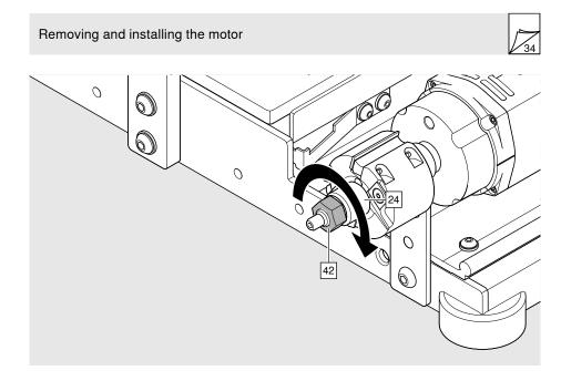
> Turn the nut [42] clockwise using the IM spanner.
