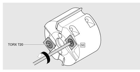
> Loosen the pre-cutter screw [50] by turning it counter clockwise.
