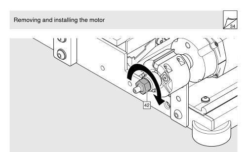
> Turn the nut [42] clockwise using the IM spanner.
