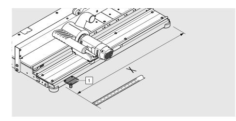
Position the fixing board [1] within the table length and screw to the frame.
