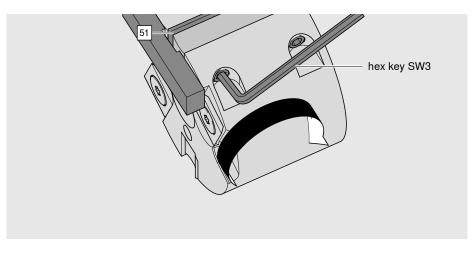
> Tighten the screw for the cutting insert [51] by turning it clockwise.
