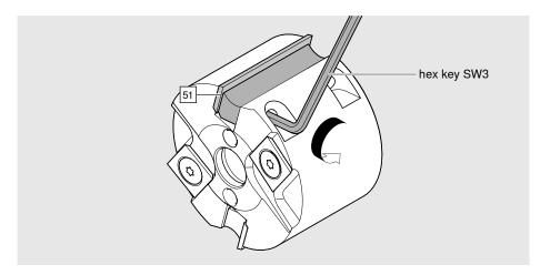
> Loosen the screw for the cutting insert [51] by turning it counter clockwise.
