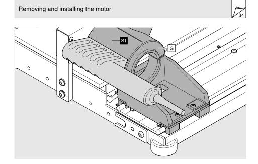
> Remove the wood chips from the housing [G].
