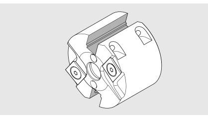
> Clean the base of the cutting inserts [51] using a dry cloth.
