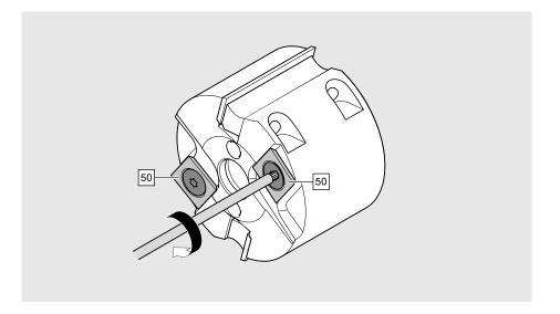
> Tighten the screw in the pre-cutter [50] by turning it clockwise.
