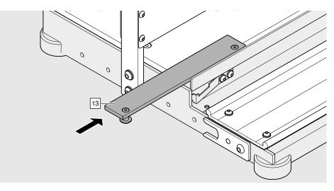
> Push the stop bar [13] into the runner of the bottom router.
