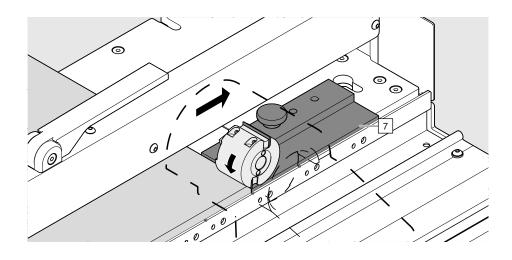
The wood stop [7] prevents torn edges and edge bands. When processing backs, the use of the wood stop [7] is strongly recommended.
