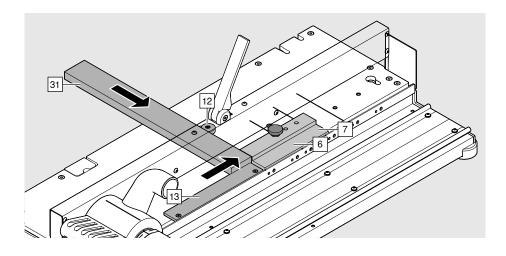
Push the back [31] onto the stop bar [13], support stop [12] and stops [6] [7], as shown.
