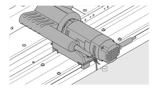
The carriage of the bottom router is secured for transport. > Remove the transportation lock [11].
