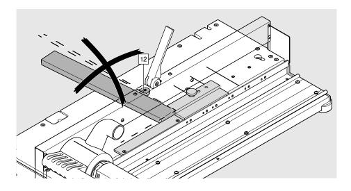
The support stop [12] must be aligned.Check whether a right angle is present.
