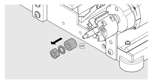
> Remove the spacer sleeve [24].
