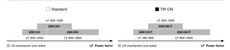
Note: the power factor is doubled when used on both sides.
