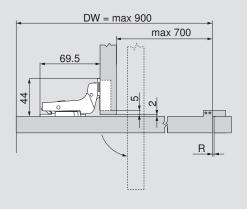
Hinge dimensions based on factory setting (mounting plate spacing = 0)
