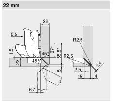
Hinge for dual applications Standard mounting plates with 0 mm spacing
