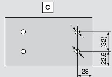
Cutting dimensions for 16 mm chipboard
