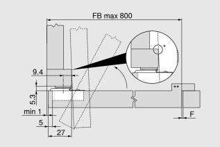
Hinge dimensions and gap calculation based on factory setting \* prevent collision
