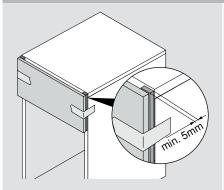
A) clamp a spacer between front and cabinet or
