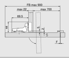
Hinge dimensions based on factory setting (mounting plate spacing = 0 mm)
