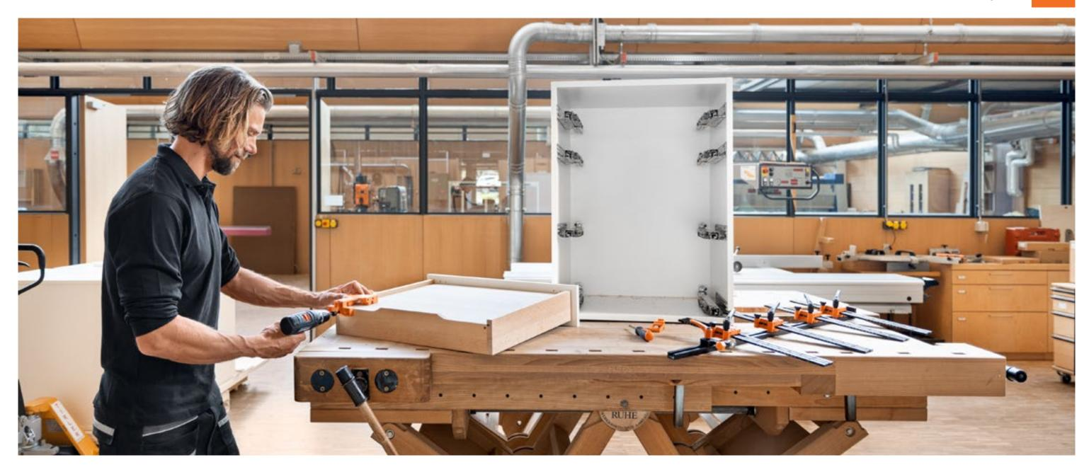
Pre-drilling allows fittings to be set even more precisely. This is particularly useful for wood and therefore also for fixing the runner profile to the drawer. You can determine the exact drilling position particularly efficiently using our drilling templates. And your work will be even easier with MINIPRESS top. If your drawers are correctly positioned on the runner profile, their feather-light glide is guaranteed.
