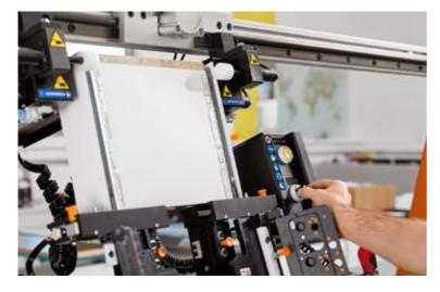
Insert the base, the cabinet back and the drawer sides. With BOXFIX plus, all parts are pneumatically fixed.
