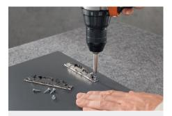
Screw on front fixing bracket in marked positions
