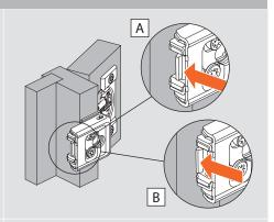
**STEP 2:** While the CLIP lever is released, pull forward on hinge to remove from cabinet.
