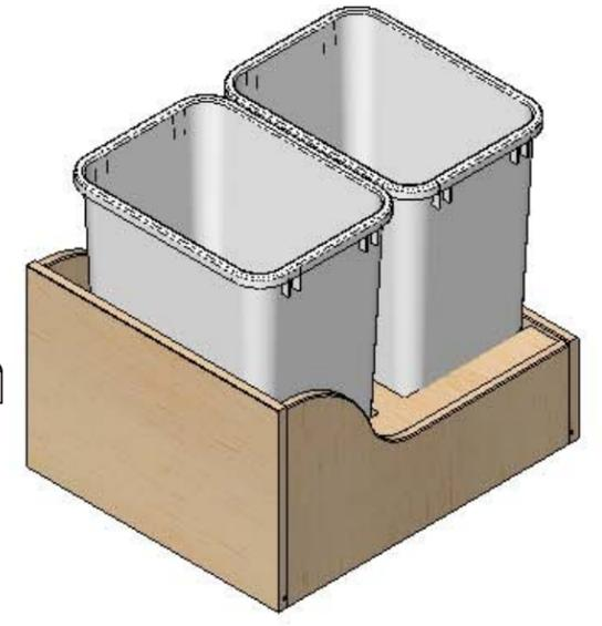
Project: Waste / recycle drawer for 21" cabinet for 18" opening width
