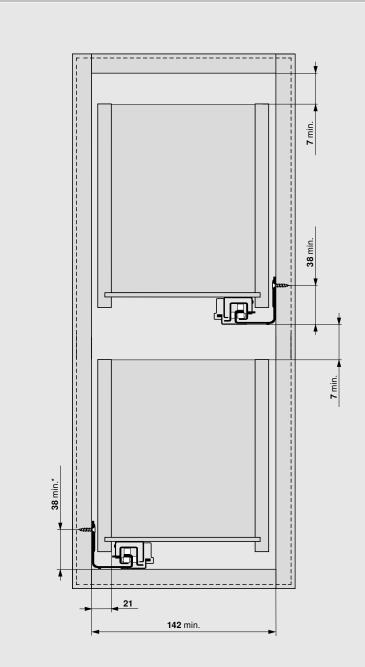
\* + 1 mm if cabinet profile is installed before cabinet assembly
