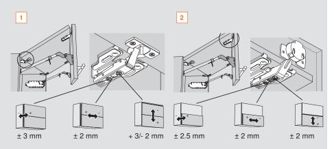
NOTE: Although not illustrated here, telescopic arm mounting plates can also be adjusted horizontally  $\pm\,2$  mm if needed.
