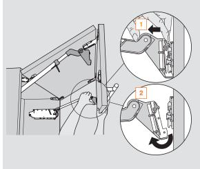
Release both arms and gently rest the top door on the loose arms. The tension will hold the doors up for the next step.
